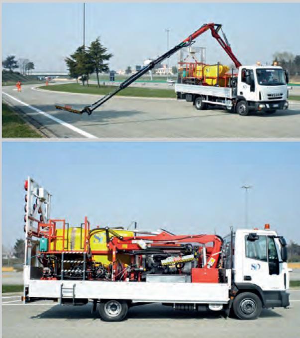
Fig. 5 – Example of special truck equipped with weed control system (Photo Sid Ambiente srl).
