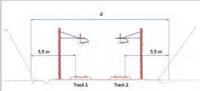
Fig. 1 – Example of the width (d) of the railway where it is necessary to ensure, according to the most common contracts, the elimination of 90% of the weeds (Italian situation).
