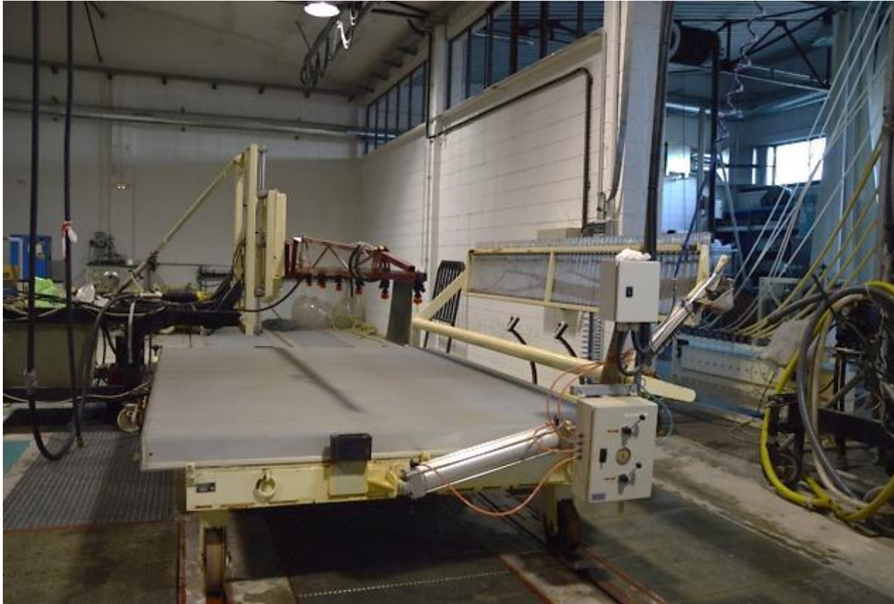
Horizontal patternator for the measurement of the traverse distribution uniformity
